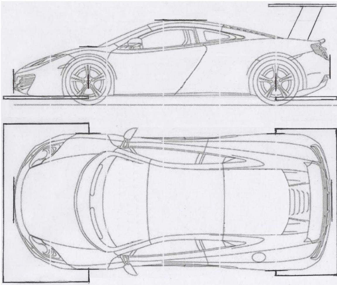
1. Front aerodynamic components may project no farther forward than 150mm beyond the forward most point of the OEM bodywork, and no further back than the front axle centerline of the vehicle.
